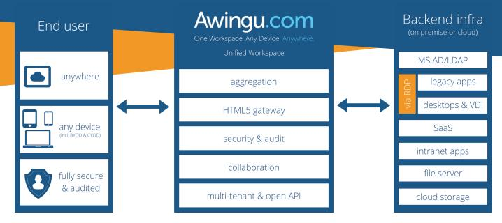
Awingu is non-intrusive and builds on top of your current architecture. It is deployed as a virtual appliance on all common hypervisors and will connect with standard protocols to your existing IT assets (e.g. RDP, WebDAV, LDAP, ...). For end users, everything is available in a browser via Awingu's online workspace. No need to install agents, plug-ins, etc.
